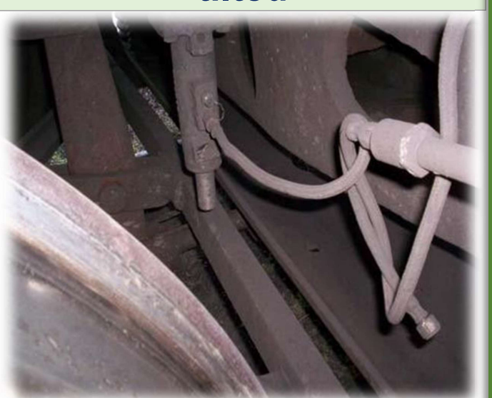
Nipples found broken on the LSD
