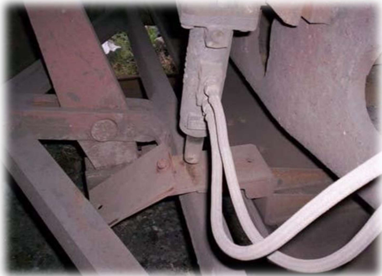
Z-plate found deformed & position shifted
