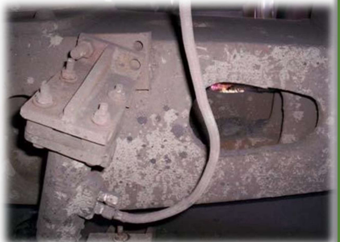
LSD mounting bracket tilted
